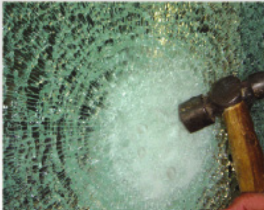
XDS (GPS) after multiple hits from a hammer*
